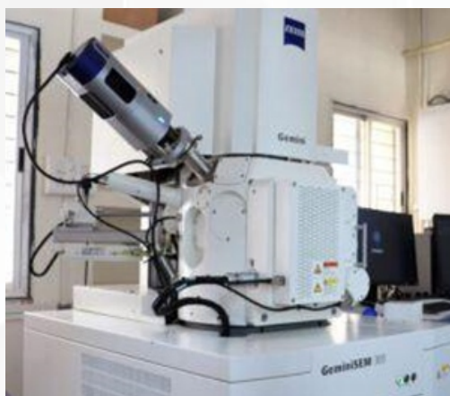
Instrument Model: Carl Zeiss GEMINISEM300
