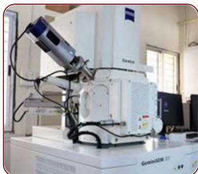
Instrument Model: Carl Zeiss GEMINISEM300
