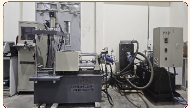
Computer controlled large direct shear test apparatus
