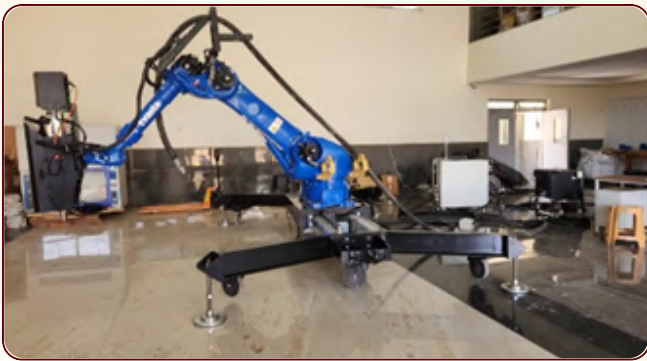
Large scale Robotic arm 3D Concrete printer
