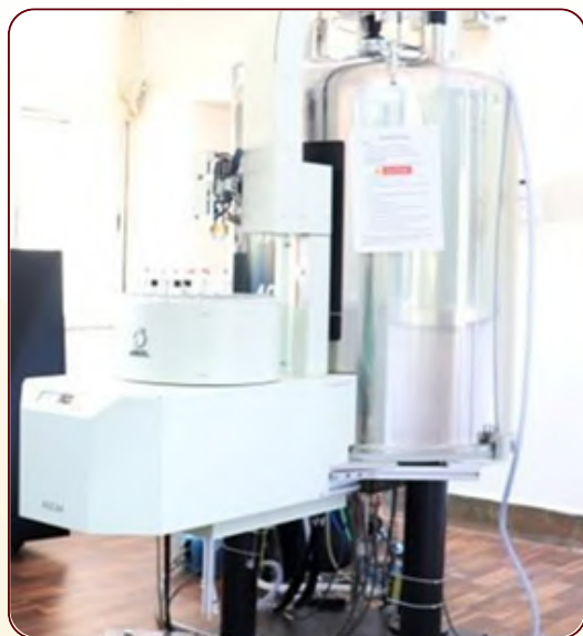
Instrument model: Jeol 400 MHz NMR spectrometer
