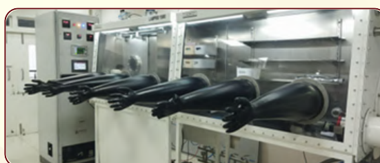
Inert Gas Workstation, LabPro 1500, Integrated Thermal + E-Beam Evaporator, RANVAC Technologies, Bengaluru, India
