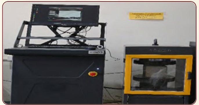
Automatic Compression Testing Machine, 3000 kN Capacity with touch panel (displacement controlled)
