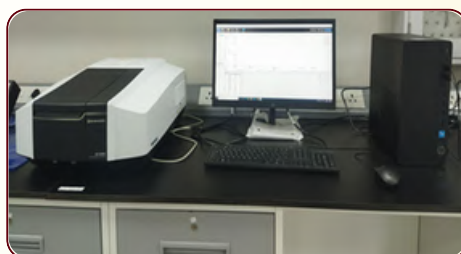
UV-Vis Spectrophotometer 2600i, Shimadzu, JAPAN
